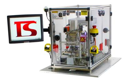
Wire Termination Analysis of Consistency and Detection of Weld Failures
